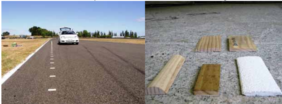
Figure 1 The test car next to a line of test blocks on the Manfeild race track and a selection of four wooden test blocks and a thermoplastic test block that were used in the testing
