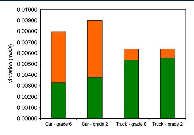
■ Vibration from road only ■ Increase in vibration over ATP markings
