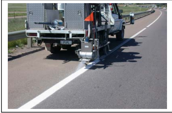
Above: Potters application equipment, used to apply the waterborne 3427 Fastrack markings.
