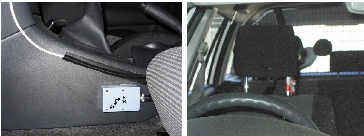
Figure 4 In-vehicle positions of accelerometer and sound level meter
